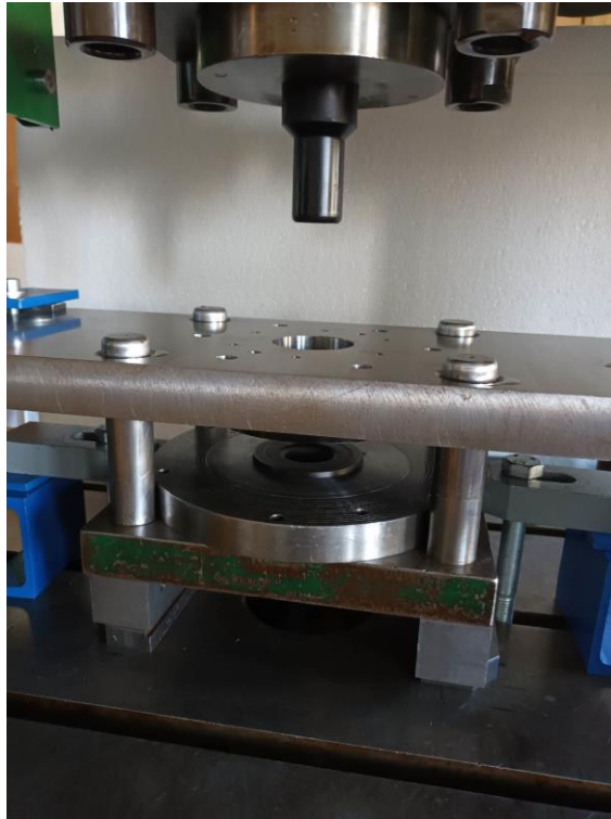
Figure 3. Deep drawing tool with polymer elements
