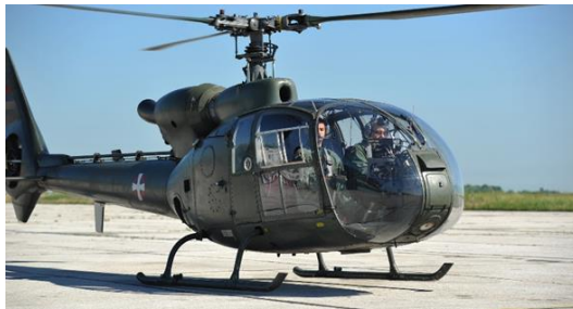
Figure 4. Landing of helicopter Aerospatiale Gazelle SA 341H at the moment of initial touchdown of backward end of right skid tube of landing gear.
