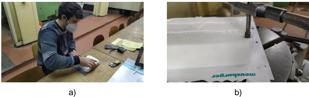
Figure 3. a) Tapping technological threads and b) grinding of the support surfaces
