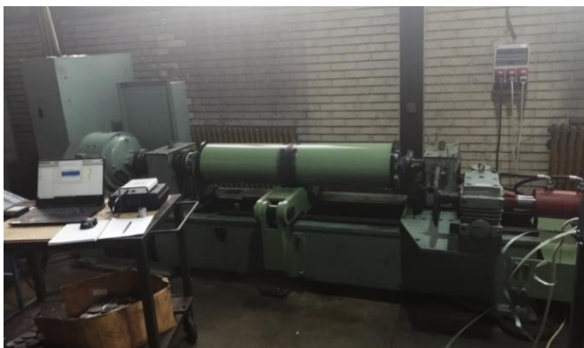
Figure 2. Experimental analysis for bearing FKL LSQFR 308
