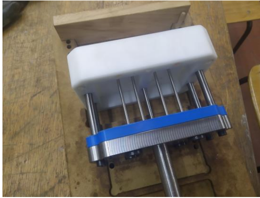
Figure 4. Assembling the ejector with the mold
