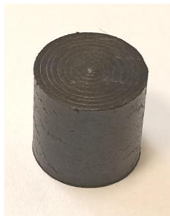
Fig. 2. Schematic and photo of the iglidur X sample
