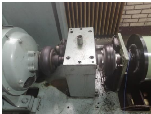
Figure 1. Schematic of the experiment for determination of bearing vibration
