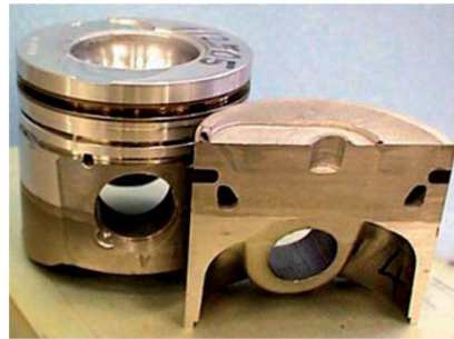
Fig.2 Friction stir processed piston [22]
