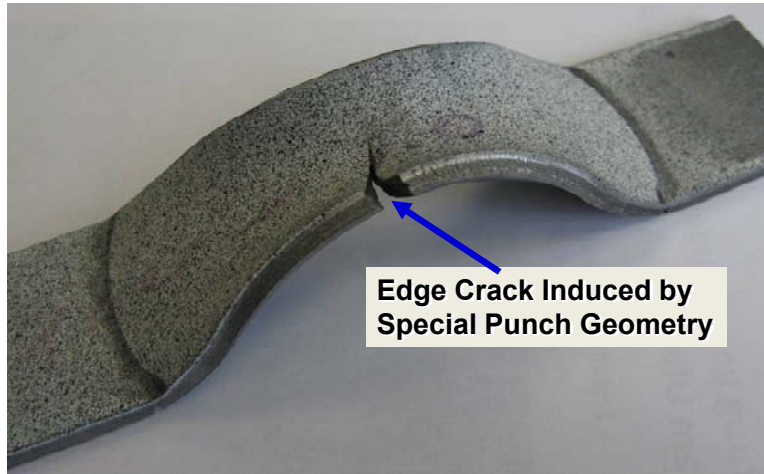
Fig. 7 New developed »Diabolo-Test« (Source: IFU/Held)
