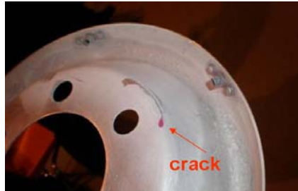
Fig. 4 Penetrant nondestructive testing method
