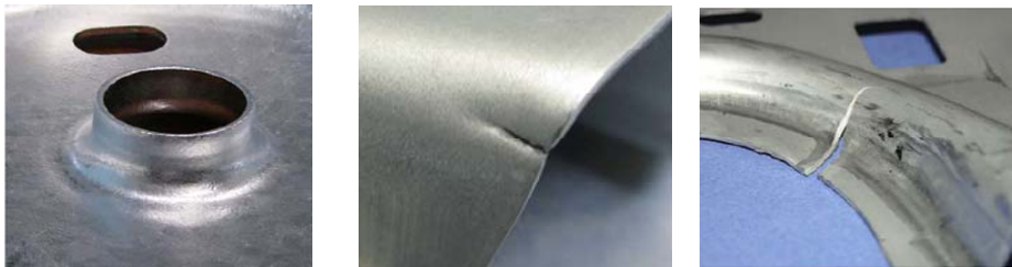
Fig. 5 Cracking of sheared edges (Source: Audi AG)
