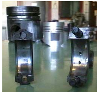
Fig. 3 Damages on connecting rod of piston
