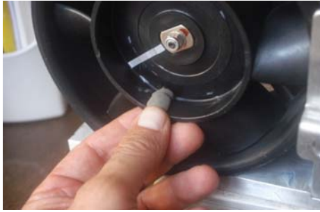
Fig. 9 Trial weight placement on the rotor
