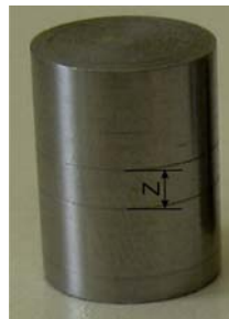
Fig. 2 Initial shape of cylindrical billets \varnothing 18 \times 24 \text{ mm}
