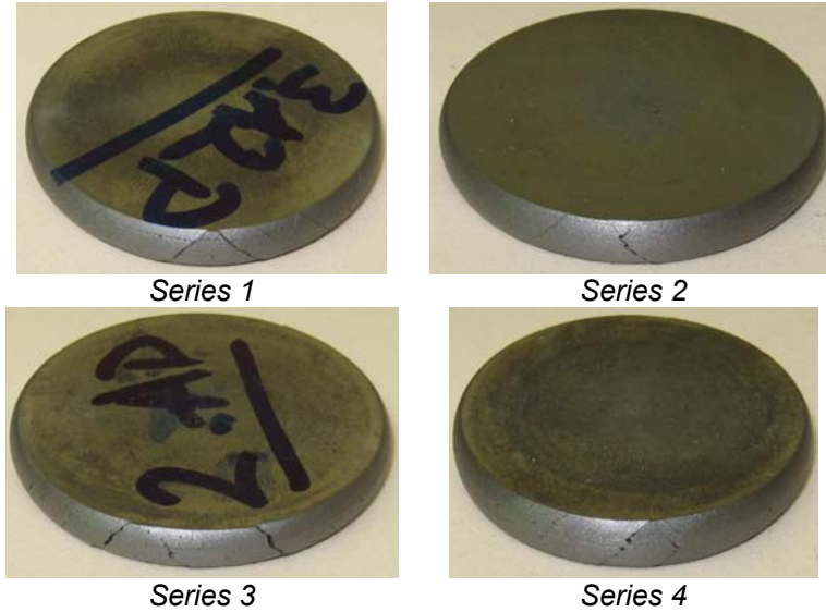
Fig. 4 Billets after upsetting processes
