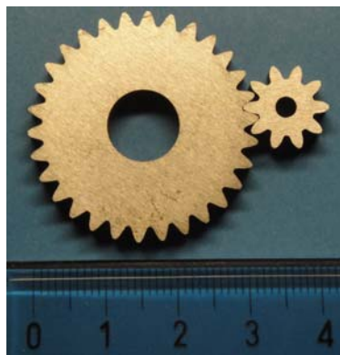
Fig. 14 S-gears defined from the rack profile material: alloy steel, z_1=10 , z_2=30 , m=1 mm
