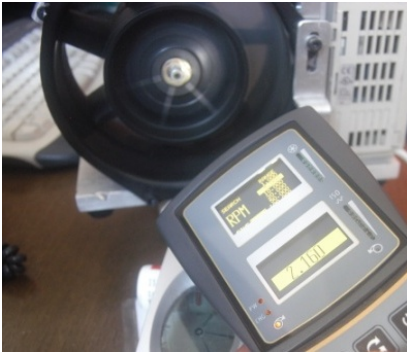
Fig. 5. Improper strobe frequency
