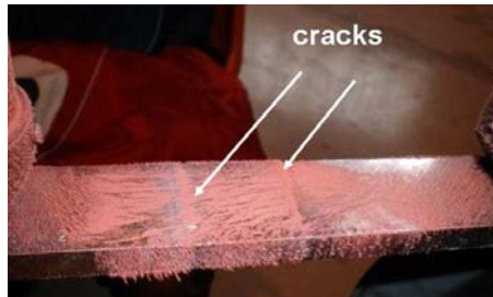
Fig. 6 Magnetic particle nondestructive testing method
